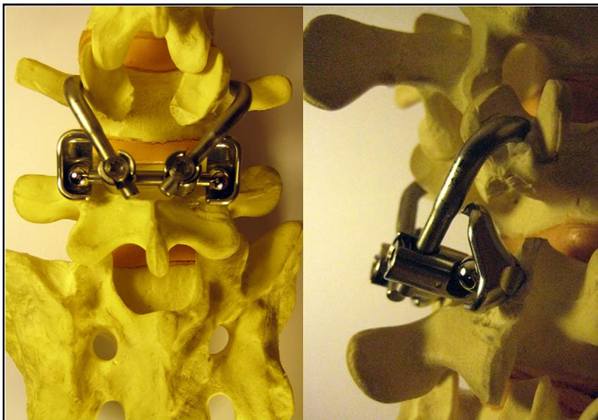
Fig. 1. Total facet arthroplasty system on a foam spine model.
