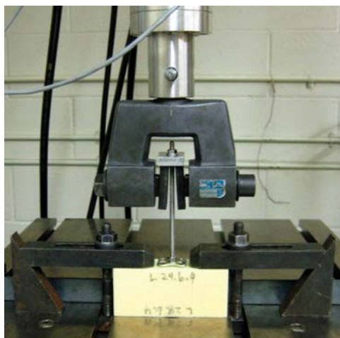
Fig. 1: Pull-out test setup. PU foam block with ALIF plate affixed by screws and secured by clamps. Threaded rod was inserted into center hole of ALIF plate to ensure uniform axial load
