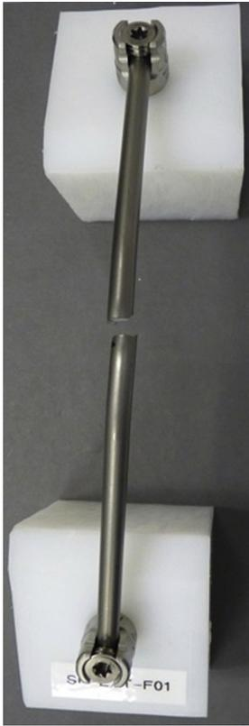
Fig. 7. The mode of failure of the single-rod group. The rods broke at the apex.
