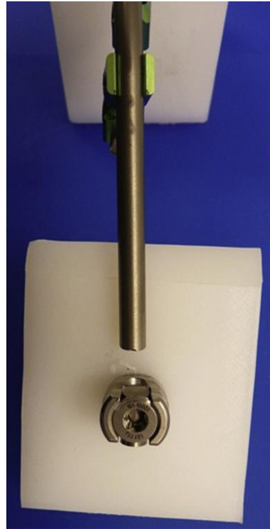
Fig. 9. The mode of failure of the bridging-rod group. The rods broke at the rod–pedicle screw junction.
