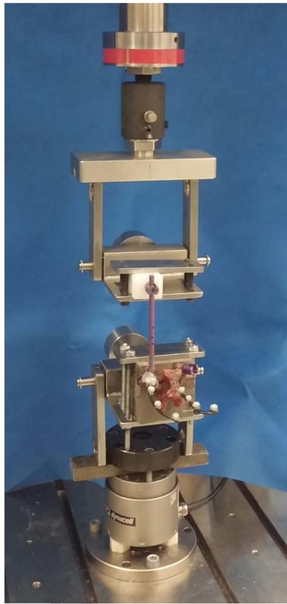
**Figure 4:** Pullout testing setup. The adjustable vice held the specimens such that the screw would be oriented vertically. A curved spinal rod was secured to the screw head. The rod was attached to top clamp via the steel wire.
