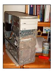
I like to start by sucking out all the dirt, hair, and dust with a vacuum. Do an extra good job around any ventilation locations as they will help to keep a steady airflow thereby keeping your internal components cooler.
