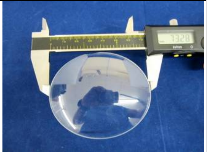
ⓘ Ex. Lens diameter is too wide and will not fit into holder of impactor
