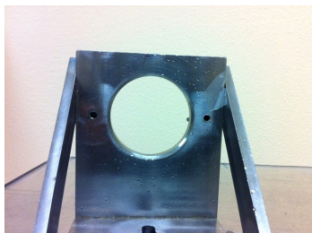
Fixture that holds test lenses that are edged round with a uniform 115^{\circ} \pm 5^{\circ} included angle bevel to a diameter 55.0 mm +0.04 mm/ -0.25 mm (2.17 + 0.002/- 0.01 in.)
