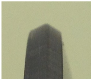
Uniform 115^{\circ} \pm 5^{\circ} included angle bevel (V bevel)
