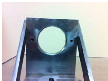
Fixture that holds test lenses that are edged round with a uniform 115^\circ + 5^\circ included angle bevel to a diameter 55.0 \text{ mm} +0.04 \text{ mm}/-0.25 \text{ mm} ( 2.17 + 0.002/- 0.01 \text{ in.} )
