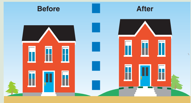
Regrading of elevated building.
