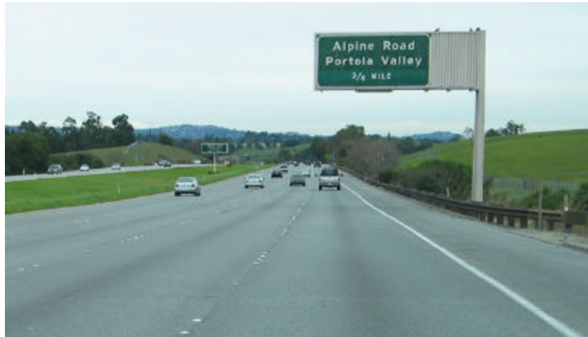
Figure 4-10: Overhead road sign that would lead to a partial satellite blockage
