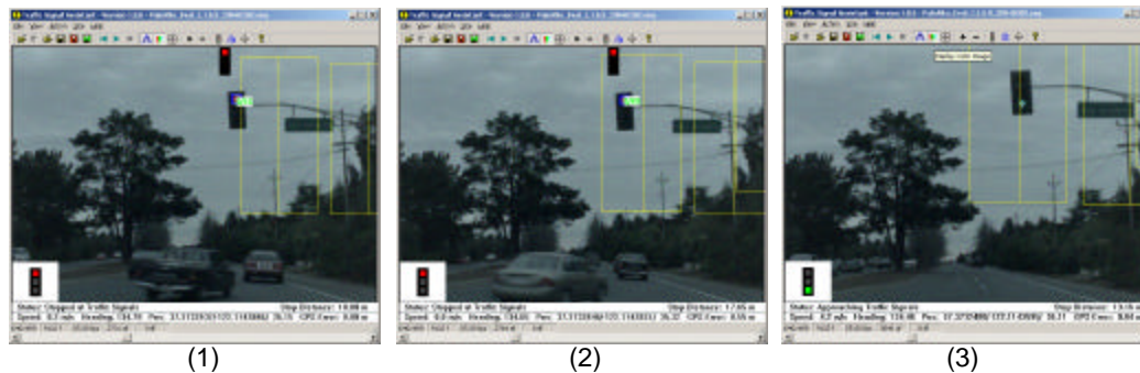
Figure 2-28: Effects of GPS error on signal search boxes
