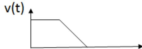
Note: Acceleration value could be achieved using driver expertise, cones to denote start and stop of braking, or dash-mounted accelerometer.
