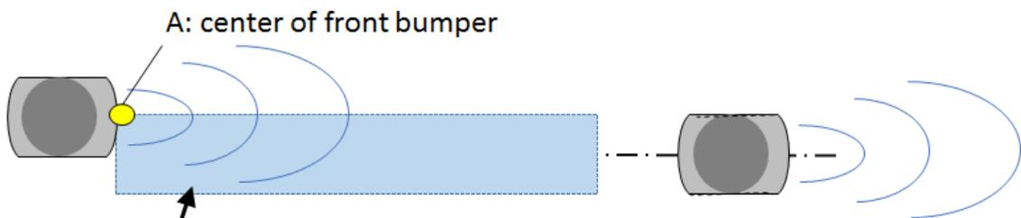
Host driven to vary headway time gap and lateral position to get various radar views of lead vehicle. Point A on host should be positioned at various points in this zone.
