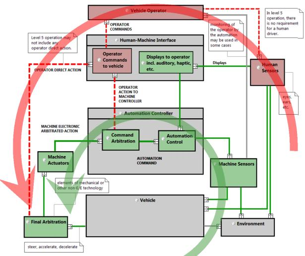
Figure 9: Control Structure for Level 5 Driving Automation
