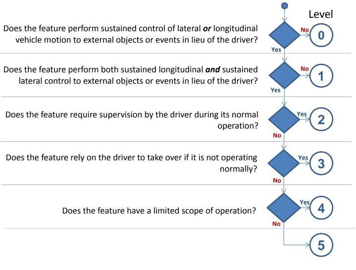
Figure 4: Flow Chart Illustrating the Methodology for Classifying Automation Features to Levels of Automation
