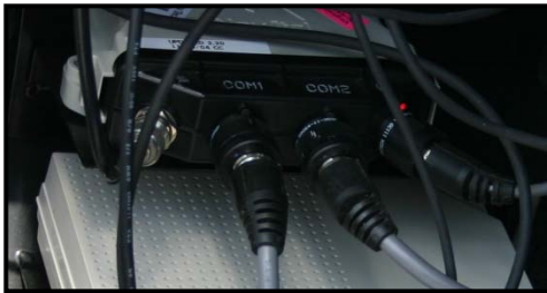
Figure 10 Novatel DGPS unit and Pacific Crest radio unit.
