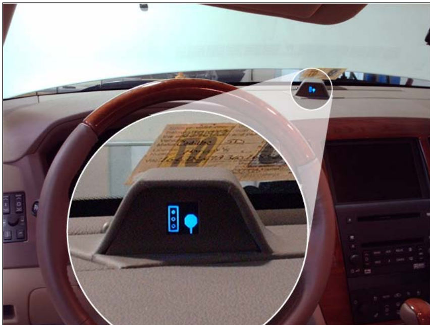
Figure 4 High-heads-down visual display LED screen.
