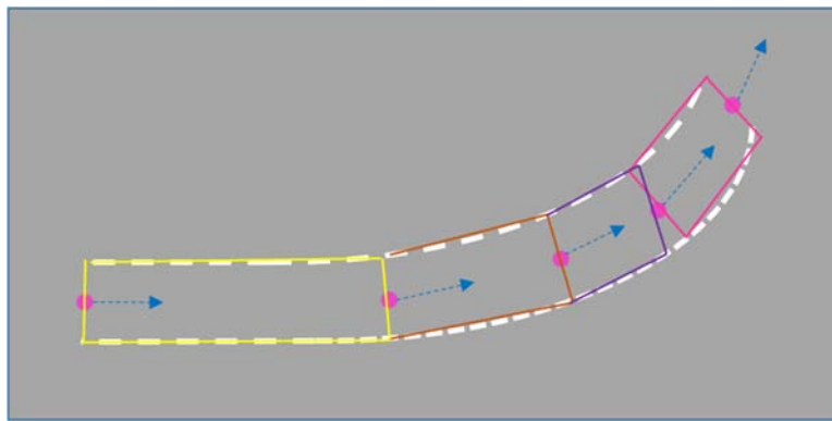
Figure 7: Lane Geometry Waypoints Based on Variable Distance
