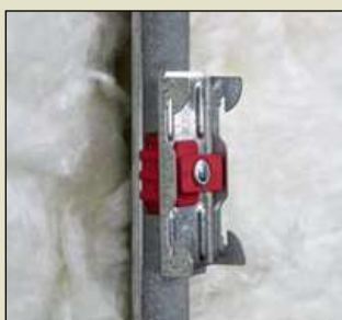
Install on metal using #10 x 1 5/8" self-tapping screw
