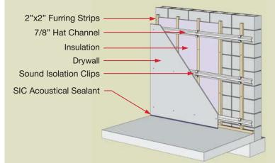
Sound Isolation Clips are the best value for proven, reliable soundproofing results in any wall or ceiling application. Call us today for a quote on your job (888) 666-5090
