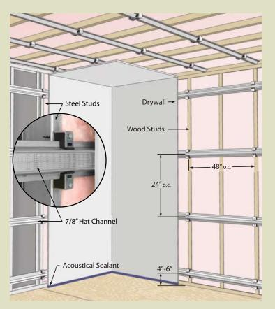
Kinetics IsoMax Clips are the easy and economical way to decouple your wall and ceiling to increase performance without the cost of staggered or double stud wall construction. Benefits include higher STC and IIC results at a lower installed cost and elimination of short circuit risk.
