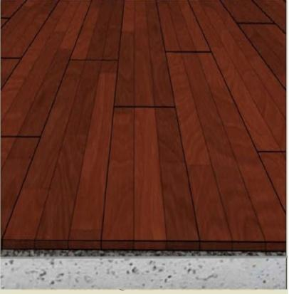
PHWU under nail down hardwood floors to reduce footstep noise to the rooms below. At only 1/8" thick PHWU will not affect transitions.
