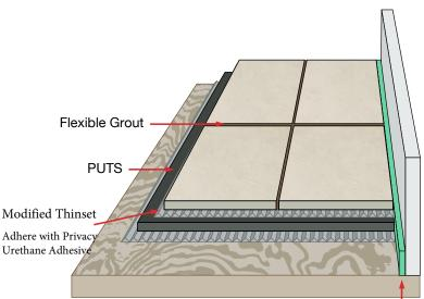
Trim PPG level with finished floor, do not grout, install baseboard
