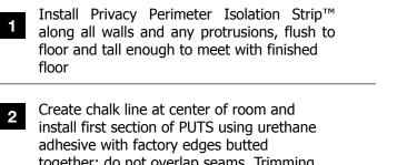
together; do not overlap seams. Trimming takes place at walls. Apply only enough Privacy Adhesive to cover area that can be worked in 20 minutes.
