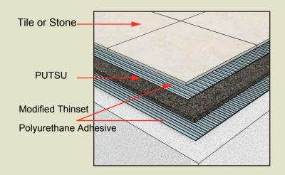
Privacy Ultimate Tile/Stone Underlay<sup>™</sup> is applied with urethane adhesive. Finished floor is installed directly on the underlay with modified thinset- no CMU required.
