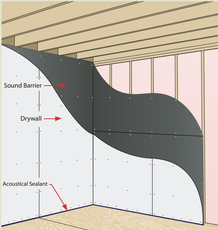
By attaching Soundproof Barrier FF directly to the studs, before drywall, noise energy will be absorbed, lowering the sound levels in the adjacent space.
