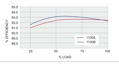
The efficiency of the compact DiamondPlus® 1100 Series peaks at over 93% at a nominal operating range.
