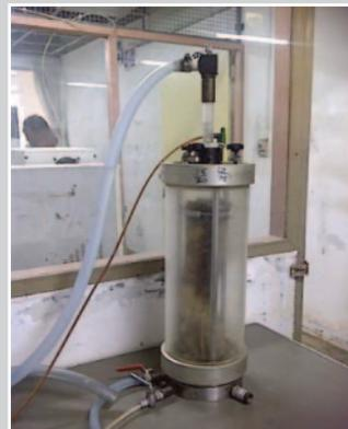
*Modified Discharge Capacity Tester*
