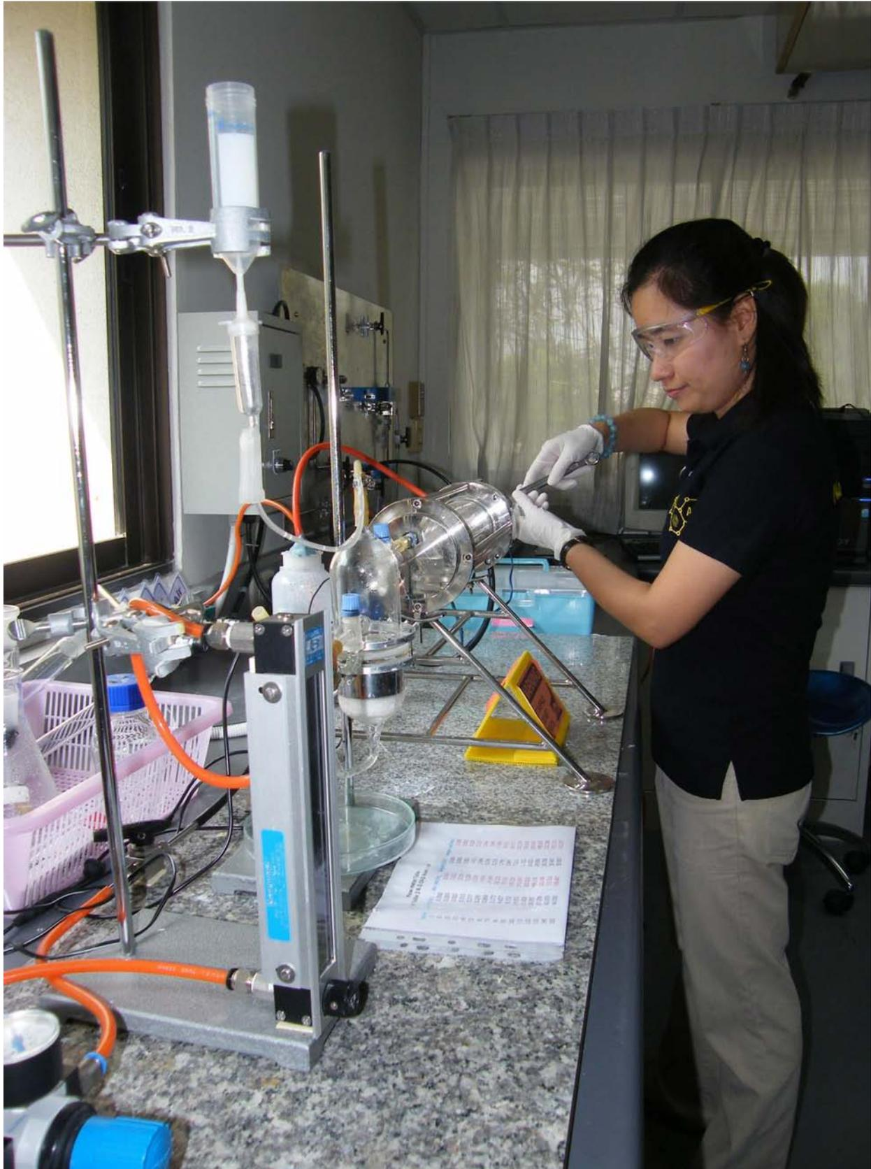
*Activities at the Center of Excellence in Nanotechnology AIT include, but not exclusively, research and development focused on the application of nanoparticles, nanomaterials, devices and sensors such as synthesizing conductive coatings of zinc oxide with fluoride for solar cell applications (shown above).*
