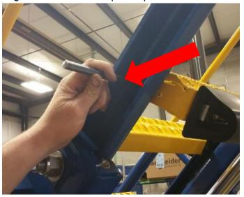
4. Drill out holes using the step drill provided until holes are opened up to  $\frac{1}{2}$ " diameter.
