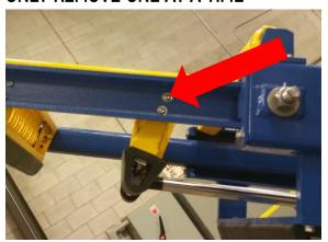
3. Align holes with the tapered punch
