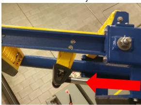
2. Remove the **upper most** bolt and nut from the frame.
