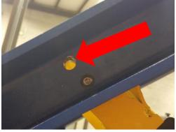
5. Insert bushing with the provided hardware, align with holes and gently tap it into position in with a hammer
