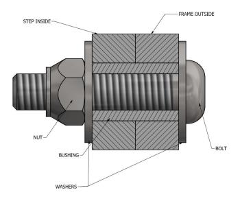
7. Repeat the process for all 4 bolts, ensuring that only one bolt is loosened and repaired at any time.
