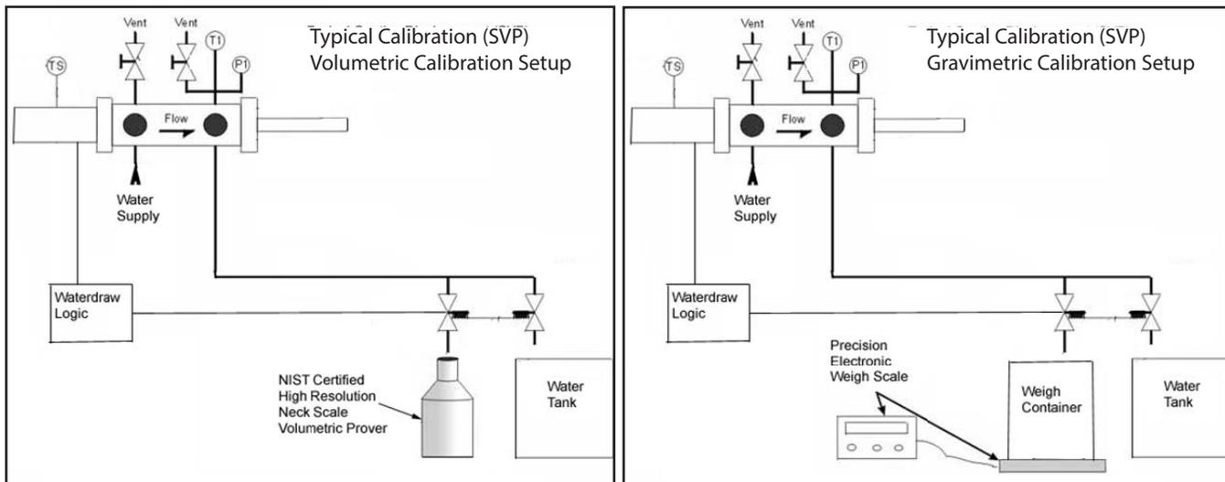
Preparation of the Prover in both cases is identical. Conducting the calibration runs is nearly identical in both cases. Gathering and recording the required data to calculate the base volumes of displacement and tank Provers is nearly identical for the volumetric method and gravimetric methods. Calculations are identical for correcting the Prover volume for pressure and temperature in both techniques.
