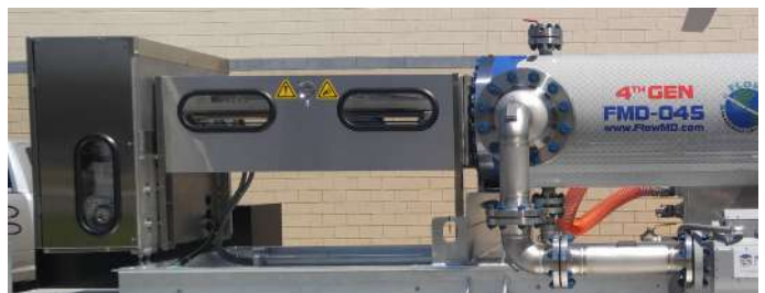
Drive end with windows on FMD-045
