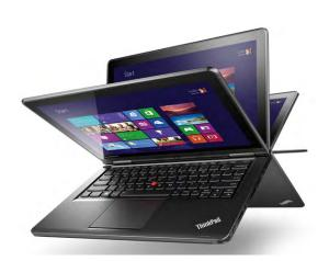
enovo ThinkPad X1 Yoga is the first convertible device with an OLED (Organic Light Emitting Diode) display and one of the lightest 14-inch laptops on the market, weighing 2.8 lbs. It features a 14" 2K (2560 x 1440) touch screen display.
