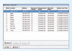
all aspects of the system. IP PBXs can be added to or removed from the group quickly. As changes are made to the group, the IP PBXs synchronize their data bases and immediately make the updated list of users available to everyone in the enterprise.
