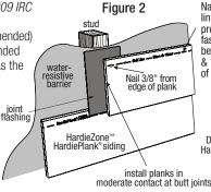
Nail line (If nail line is not present place . fastener between 3/4" & 1" from top of plank)
