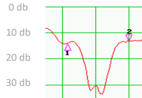
Rtn Loss > 13.9 dB at 395 to 450 MHz
