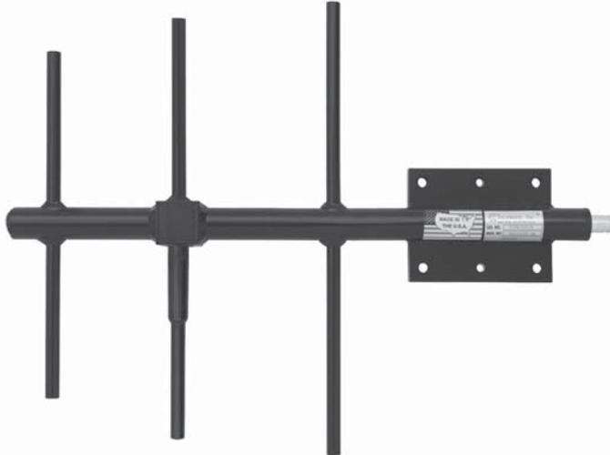
The Telewave ANT390Y5-WR is a high performance directional antenna, designed especially for point to point as well as point/multipoint applications. This antenna produces 5 dBd forward gain with an excellent front-to-back ratio. Solid aluminum elements with 360° welds prevent intermodulation and provide exceptional strength.
