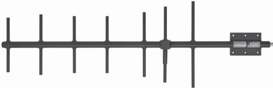
The Telewave ANT450Y10-WR is a high performance directional antenna, designed especially for point to point as well as point/multipoint applications. This antenna produces 10 dBd forward gain with an excellent front-to-back ratio. Solid aluminum elements with 360° welds prevent intermodulation and provide exceptional strength.
