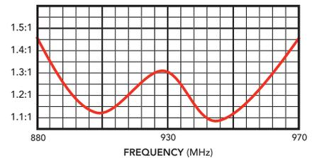
The Telewave ANT930Y10-WR Yagi is a high performance directional antenna, designed especially for point to point as well as point/multipoint control applications. Seven elements provide a minimum of 10.5 dBd (12.6 dBi) forward gain, excellent front-to-back performance, and coverage of the entire 900 MHz commercial band. The boom and elements are solid 360° welded aluminum to prevent intermodulation and provide exceptional strength.
