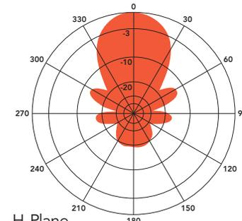
The Telewave ANT1800Y10-WR is a rugged, wideband, high gain Yagi antenna for the DCS-1800 band, designed for handheld use with many types of portable wireless analyzers. This antenna can also be installed for fixed use in any environment. The antenna uses eight solid brass elements, and produces 10 dBd forward gain with excellent front-to-back performance. Construction and design are optimized to prevent RF intermodulation, and ensure precise pattern control.
