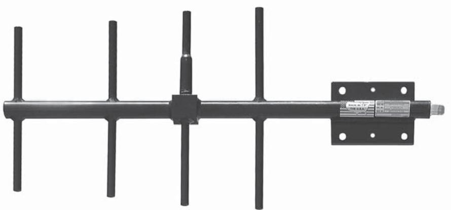
The Telewave ANT450Y7-WR is a high performance directional antenna, designed especially for point to point as well as point/multipoint applications. This antenna produces 7 dBd forward gain with an excellent front-to-back ratio. Solid aluminum elements with 360° welds provide exceptional strength and prevent intermodulation.
