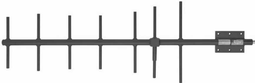
The Telewave ANT430Y10-WR is a high performance directional antenna, designed especially for point to point as well as point/multipoint applications. This antenna produces 10 dBd forward gain with an excellent front-to-back ratio. Solid aluminum elements with 360° welds prevent intermodulation and provide exceptional strength.
